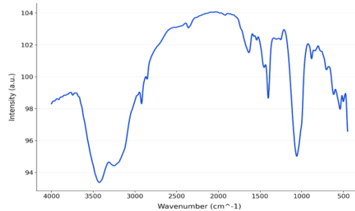
Figure 2: Fourier Transform Infrared spectrum of guava extract displaying major functional groups.
