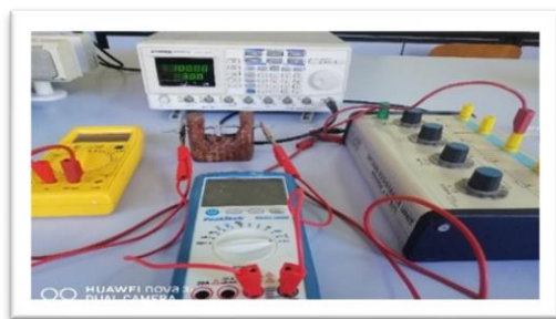
Fig. 2 Illustrates the electrical circuit employed for determining the dielectric constant.
