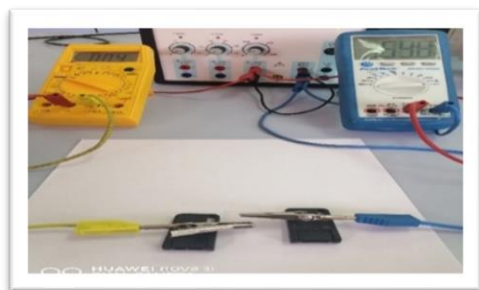
Fig.1 Depicts the electrical circuit designed for measuring electrical conductivity at room temperature.
