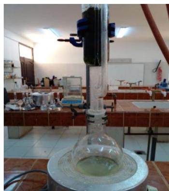
**Figure 2:** Using soxhlet extraction technique
